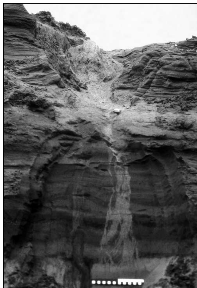
Figure 12. A complete second-generation sand wedge, with a lighter fill within a darker host rock. The view is steeply upwards, and is somewhat distorted due to closeness to the cliff face. Scale bar 20 cm. The layering that appears to cross the host and the wedge is an artefact of cutting the face back with a small trowel.
